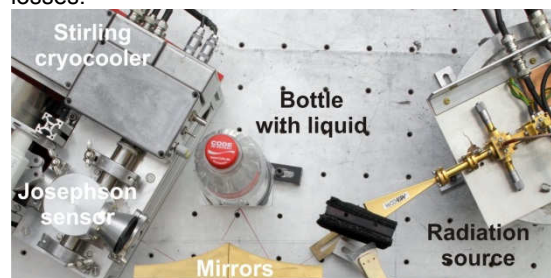
FIG. 1. Demonstrator of liquid identifier with quasioptical coupling
