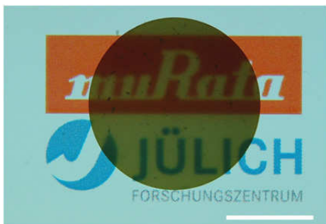
FIG. 2 Translucent 0.78 mm thick \text{BaTiO}_3 ceramic pellet containing 2 mol.% of La-addition after sintering for 2 hours at 1350 °C and subsequent annealing for 30 hours at 1000 °C in pure oxygen. The nominal composition is (\text{Ba}_{0.99}\text{La}_{0.02})\text{Ti}_{1.005}\text{O}_3 . The white bar in the right bottom corner of this image indicates 10 mm in length.
