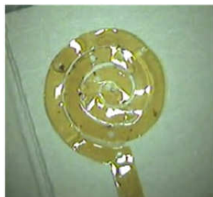
FIG. 4: A VLARS prototype with spiral design after experiments on porcine cadaver eyes.
